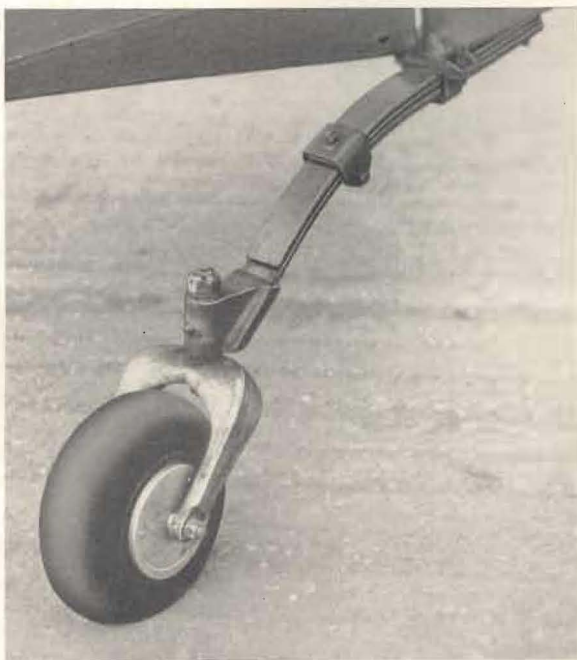
Much better taxiing characteristics result when the pneumatic tail wheel is fitted. This particular photograph shows a standard type although it can be modified to be both steerable and fully castoring.
