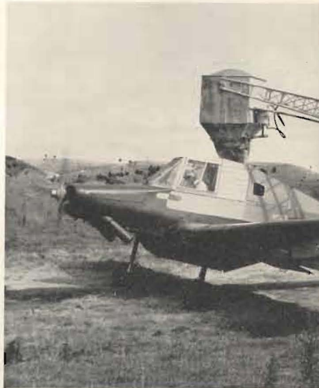
Having returned empty, the Agricola turns into wind. The driver positions the loading hopper funnel above the aircraft. Meanwhile the hopper releases the load into the aircraft. Meanwhile the driver sets his flaps at take-off position. Loading is complete and the aircraft takes-off. Total time for the
